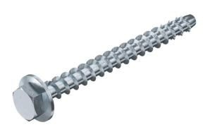
Bolt tie for direct mounting without additional anchors in cracked and uncracked concrete and masonry. With hex head drive and pressed washer to accept large loads. Suitable for fastening suspended loads from suspended supports and wall brackets in wet rooms and in outdoor areas.
