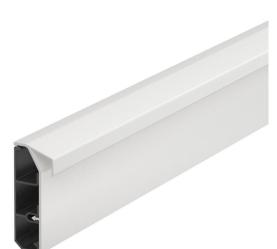
SL-T skirting trunking for covered cable routing in internal areas. The colour of the trunking bases can vary depending on the production method. With snap-on cover and base, with base perforation for direct wall mounting. Carry out a change of direction using a mitre cut and close the trunking ends with end pieces. Service outlet for mounting power and data technology. With carpet strip for a clean finish.
