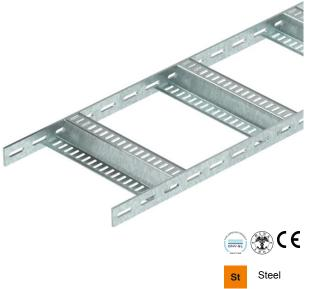
Shipbuilding cable ladder with perforated side rail of side height 40 mm with welded, perforated Z rungs. Load tested according to IEC in conjunction with connector, type SLV.
