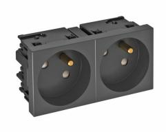
Socket with earthing pin and side connection, Double 33°, with increased touch protection, with screwless terminals, 2-pin, 16 A, 250 V $\sim$ , with connection terminals to IEC 60884-1.
