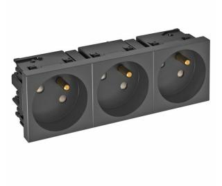
Socket with earthing pin and side connection, Triple  $33^{\circ}$ , with increased touch protection, with screwless terminals, 2-pin, 16 A, 250 V~, with connection terminals to IEC 60884-1.
