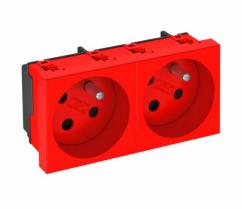
Socket with earthing pin Double 33°, encoded version, with increased touch protection, with screwless terminals, 2-pin, 16 A, 250 V $\sim$ , with connection terminals to IEC 60884-1. The socket can only be used in conjunction with an encoding pin, type CST-STD.
