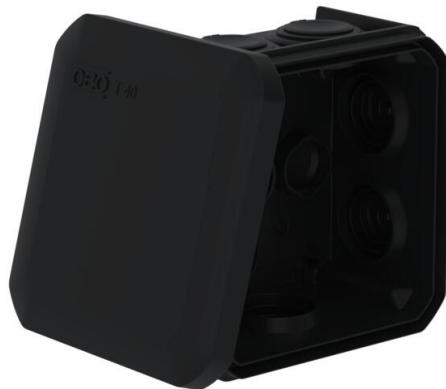
Junction box for the connection of cables indoors and in protected outdoor areas. Square design with plug-in seals to the sides and knock-out entries in the bottom. Suitable for wall and ceiling mounting and on mounting panels. With the option to fasten inside. With fixed clamping cover. Made from halogen-free, UV-resistant materials.
